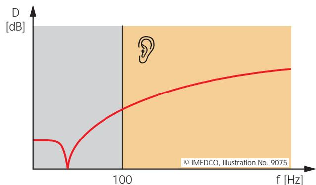
Where the mass of the floor is particularly high, it can only be excited to a small degree by MRI vibration. Single elastic supports are usually all that are needed to optimally decouple the MRI equipment from the building structure and provide adequate soundproofing in the audible range (100 Hz to 20,000 Hz).
